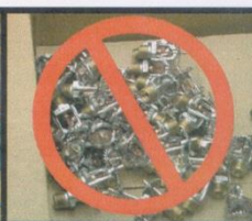
INCORRECT! (sprinklers placed loose in box)
